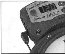
Connect the RP-2 pad to Trig 1 of the RM-2 Module
